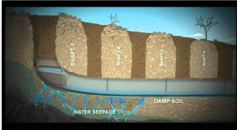
Picture 8: Illustration of a Karez system
