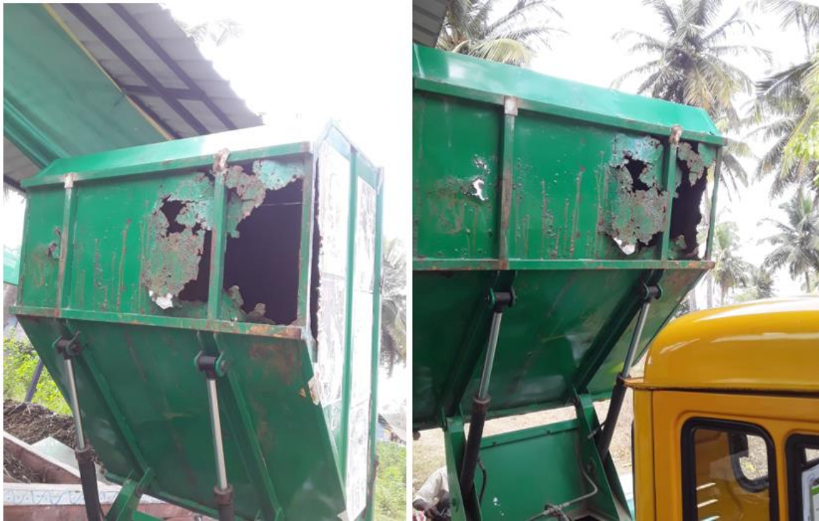
Fig 3: Broken WCV in Kudluru
